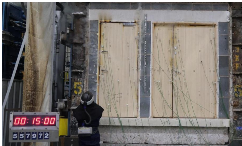
The unexposed face of the specimen after a test duration of 15 minutes
