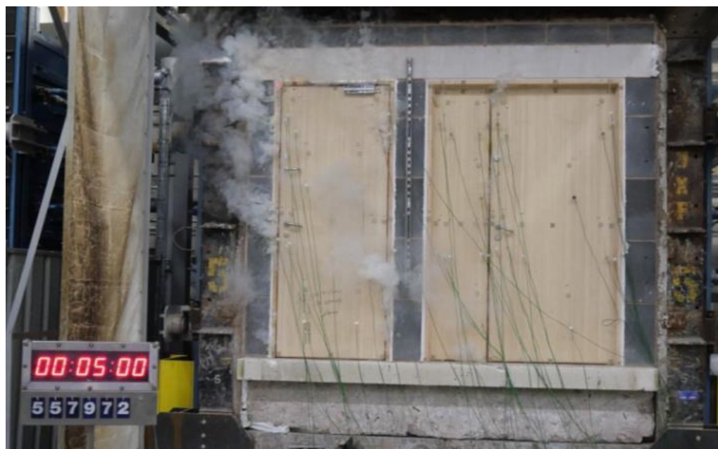
The unexposed face of the specimen after a test duration of 5 minutes
