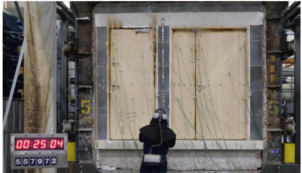
The unexposed face of the specimen after a test duration of 25 minutes
