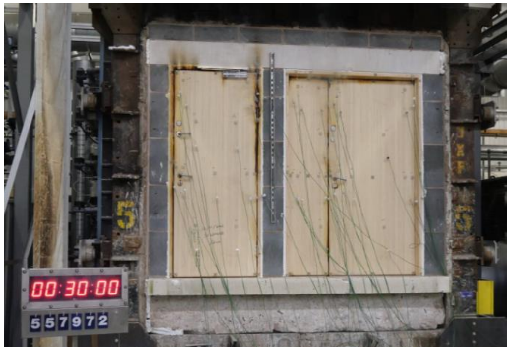
The unexposed face of the specimen after a test duration of 30 minutes
