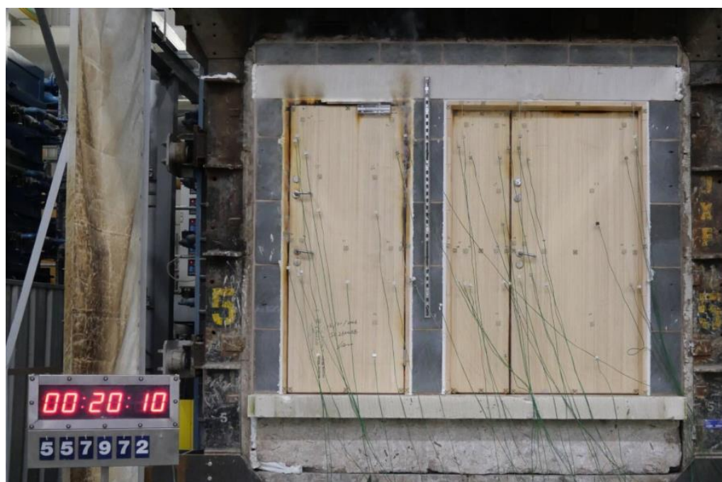
The unexposed face of the specimen after a test duration of 20 minutes
