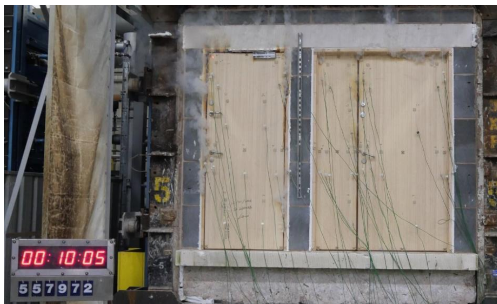
The unexposed face of the specimen after a test duration of 10 minutes
