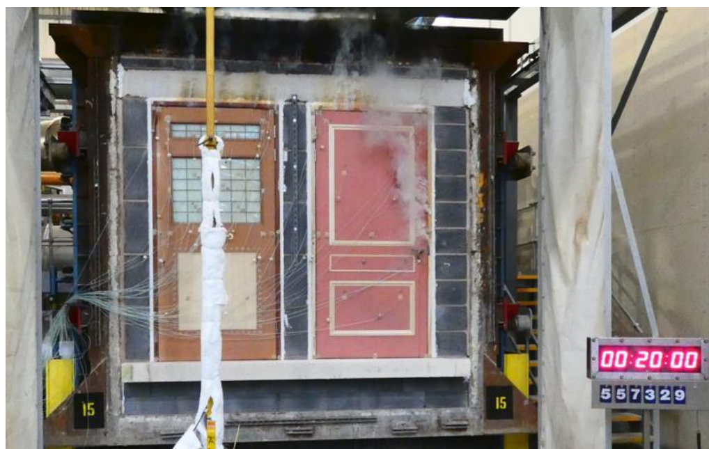
The unexposed face of the specimens after a test duration of 20 minutes
