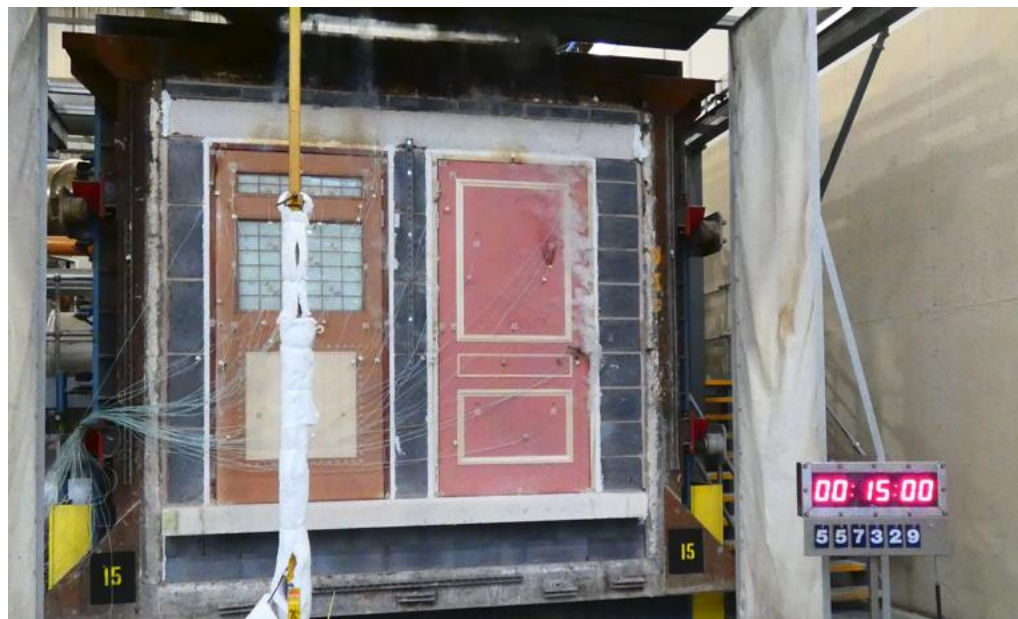
The unexposed face of the specimens after a test duration of 15 minutes
