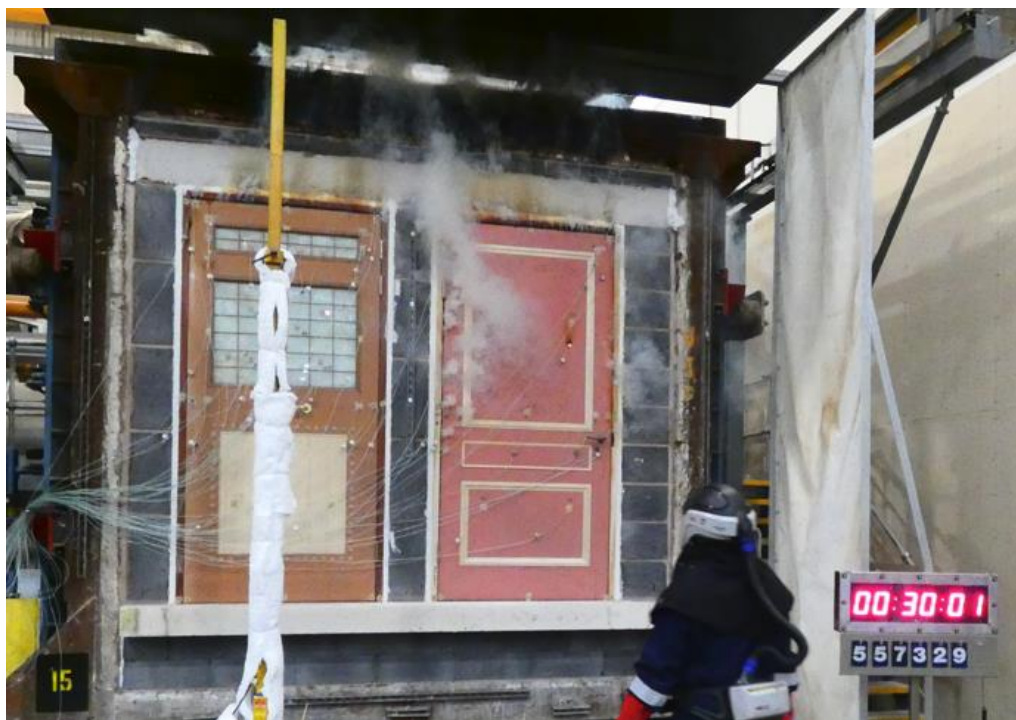
The unexposed face of the specimens after a test duration of 30 minutes
