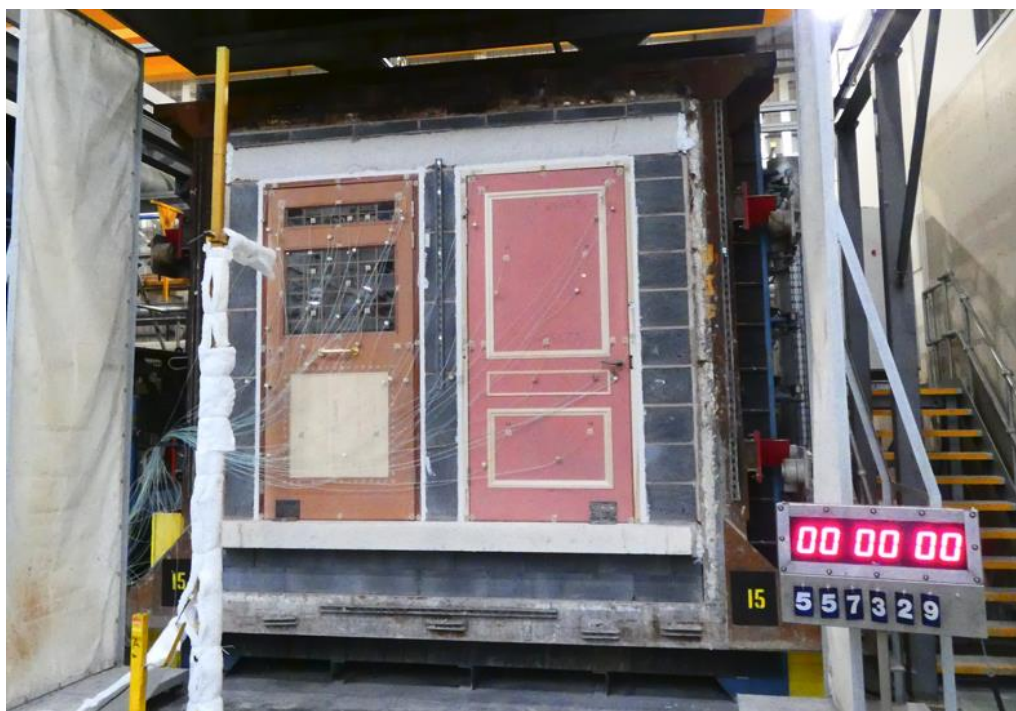
The unexposed face of the specimens prior to the start of the test
