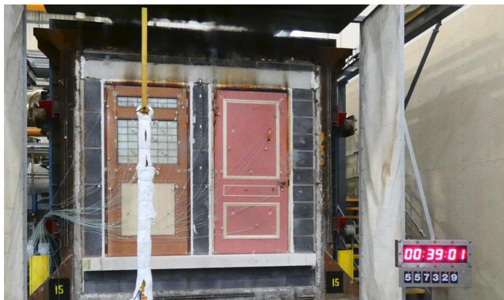
The unexposed face of the specimens after a test duration of 39 minutes
