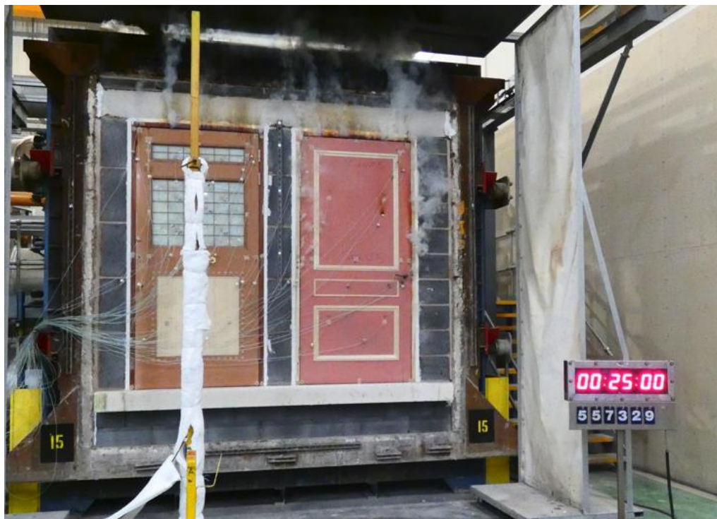
The unexposed face of the specimens after a test duration of 25 minutes
