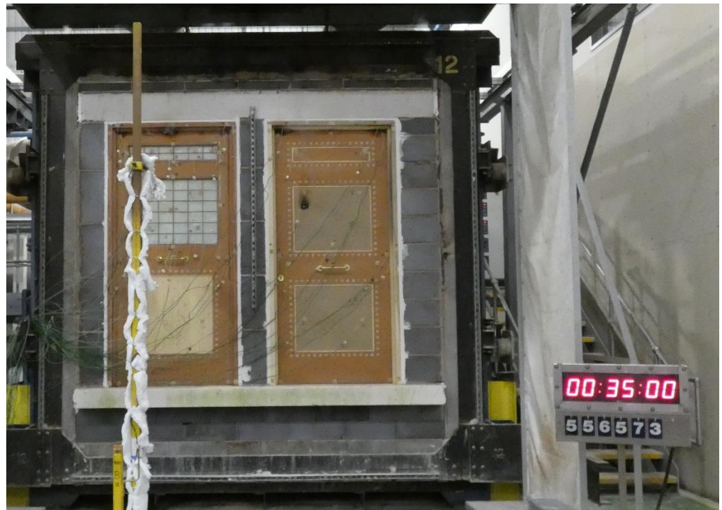
The unexposed face of the specimens after a test duration of 35 minutes
