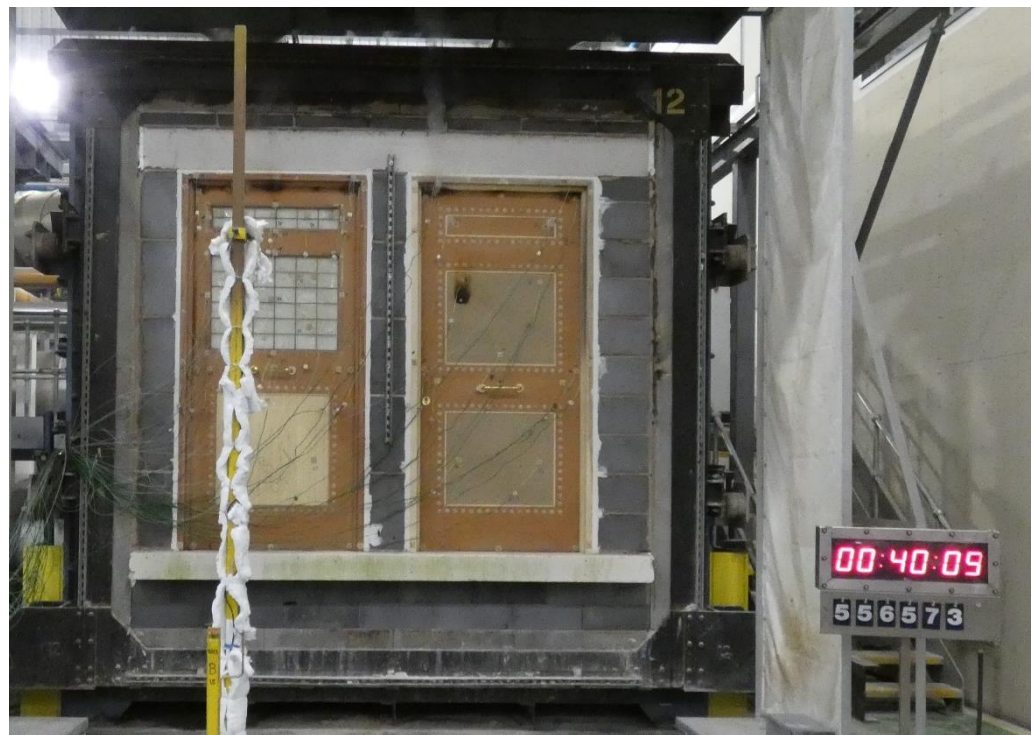
The unexposed face of the specimens after a test duration of 40 minutes
