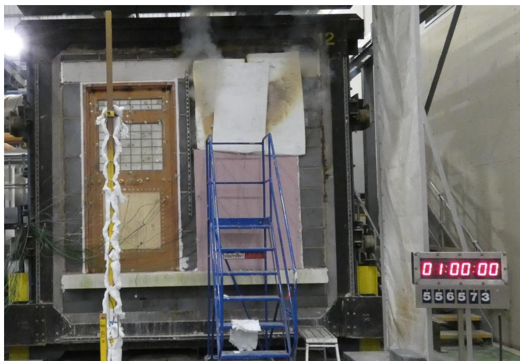
The unexposed face of the specimens after a test duration of 60 minutes
