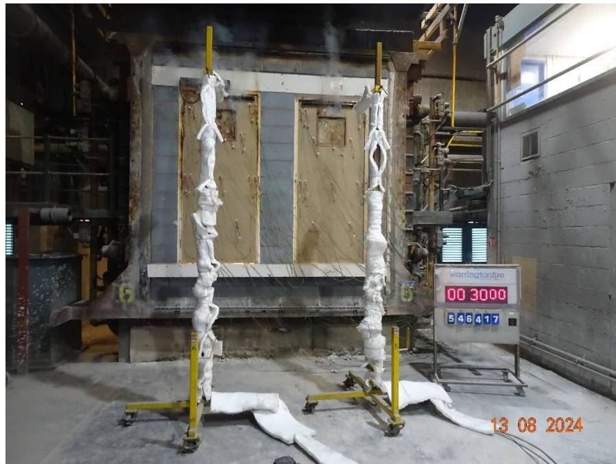
Figure 32 Unexposed face of the specimens at 30 minutes of testing
