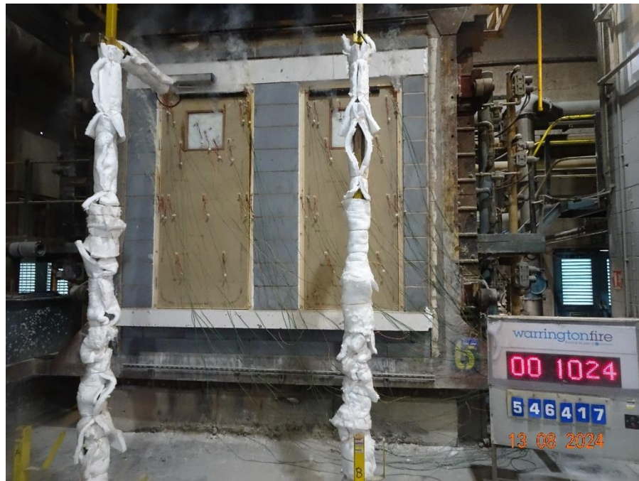
Figure 30 Unexposed face of the specimens at 10 minutes of testing
