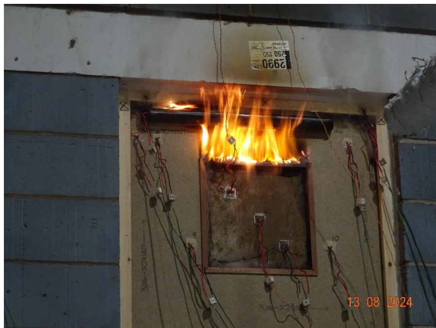
Figure 33 Exposed face of the specimen at 36 minutes 40 seconds displaying sustained flaming on Doorset B
