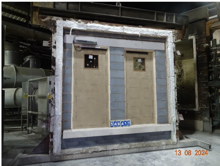
Figure 29 Exposed face of the specimens before the start of the test
