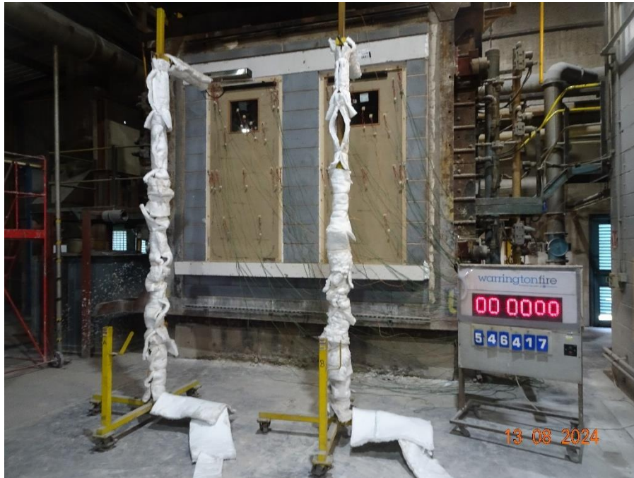
Figure 28 Unexposed face of the specimens before the start of the test
