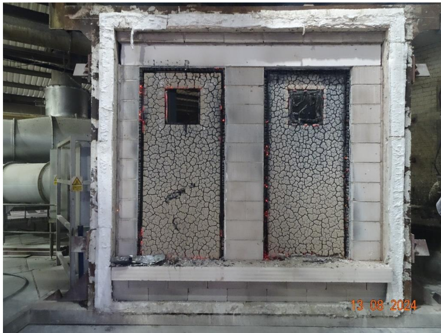
Figure 34 Exposed face of the specimens at the end of the test
