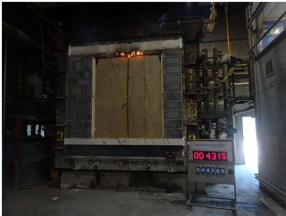
Figure 27 Unexposed face of the specimen at the termination of the test.
