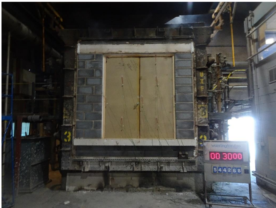
Figure 25 Unexposed face of the specimen at 30 minutes of testing.
