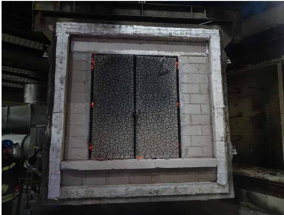
Figure 28 Exposed face of the specimen at the end of the test.
