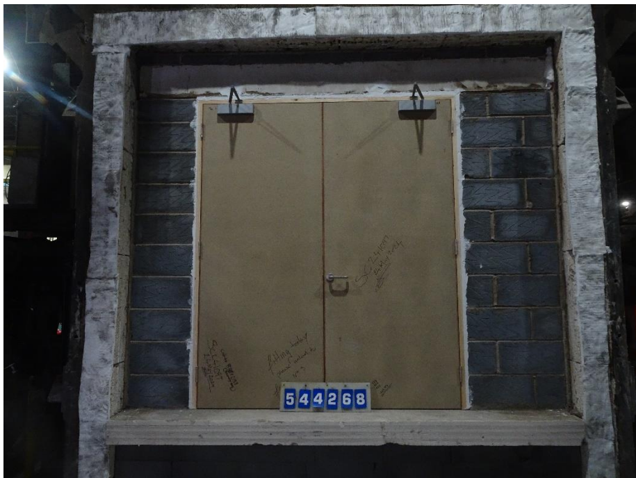
Figure 23 Exposed face of the specimen before the start of the test
