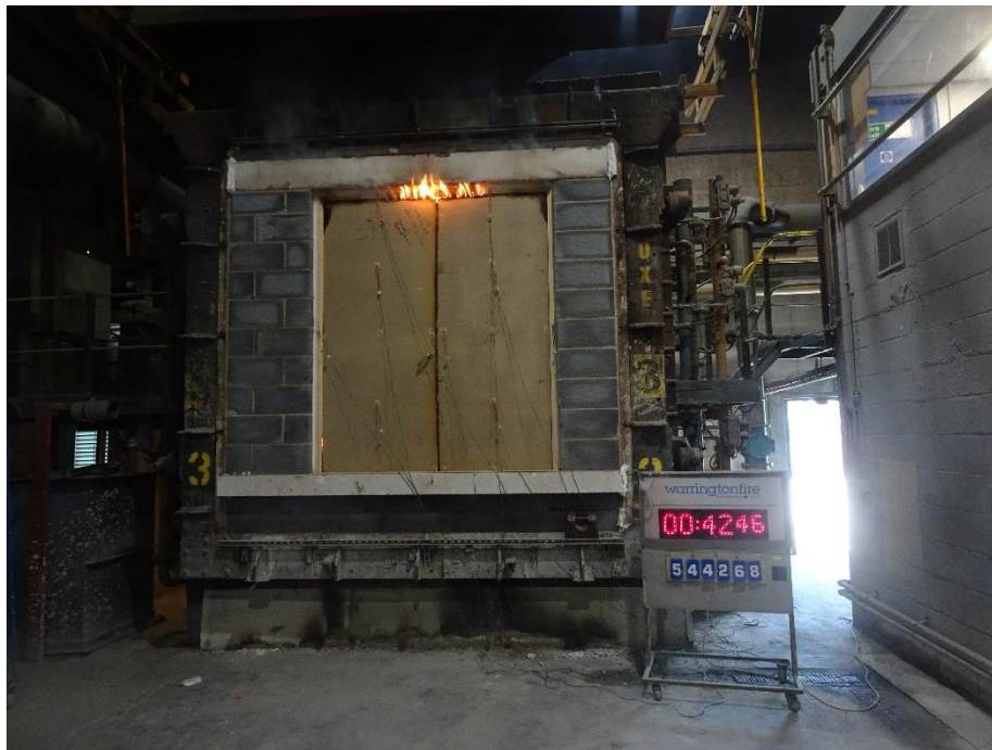
Figure 26 Unexposed face of the specimen at 42 minutes displaying sustained flaming.
