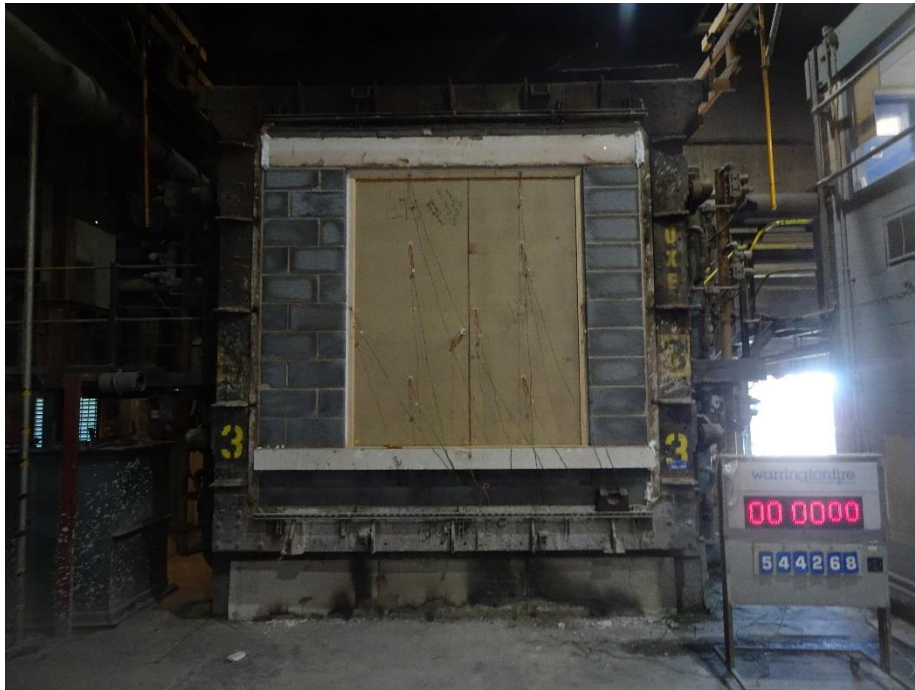
Figure 22 Unexposed face of the specimen before the start of the test
