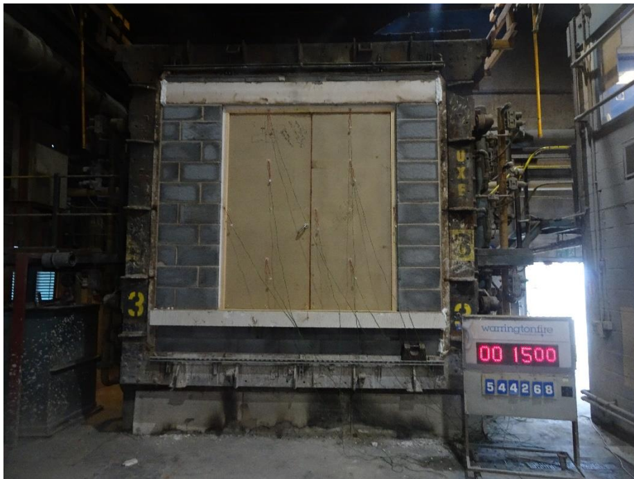
Figure 24 Unexposed face of the specimen at 15 minutes of testing.
