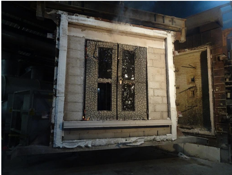
Figure 16 Exposed face of the specimen at the end of the test
