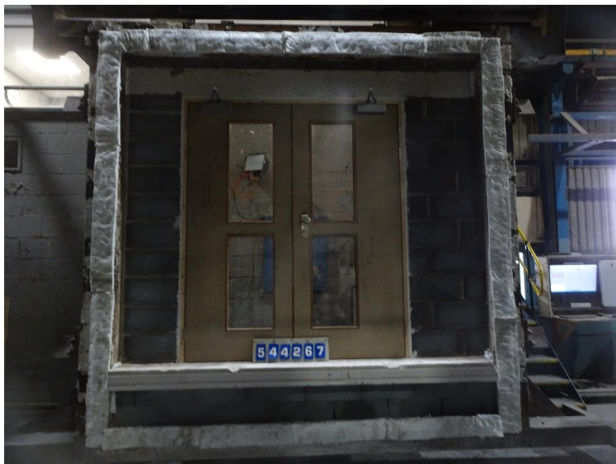
Figure 11 Exposed face of the specimen before the start of the test
