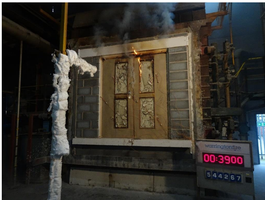
Figure 15 Unexposed face of the specimen at the termination of the test
