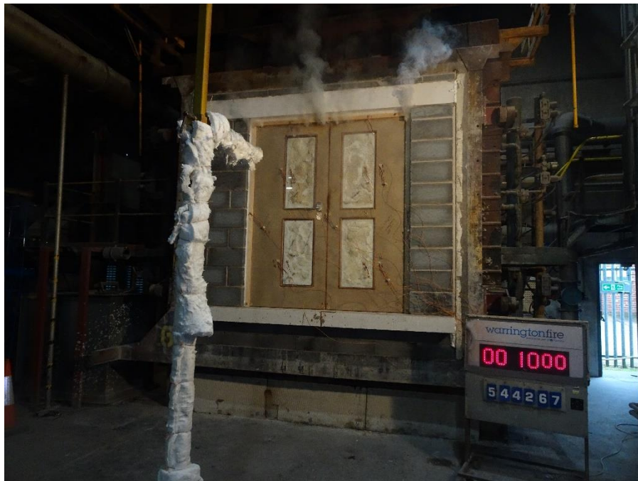
Figure 12 Unexposed face of the specimen at 10 minutes of testing
