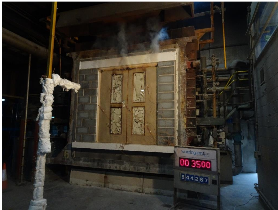
Figure 14 Unexposed face of the specimen at 35 minutes of testing when sustained flaming had occurred at the meeting edge
