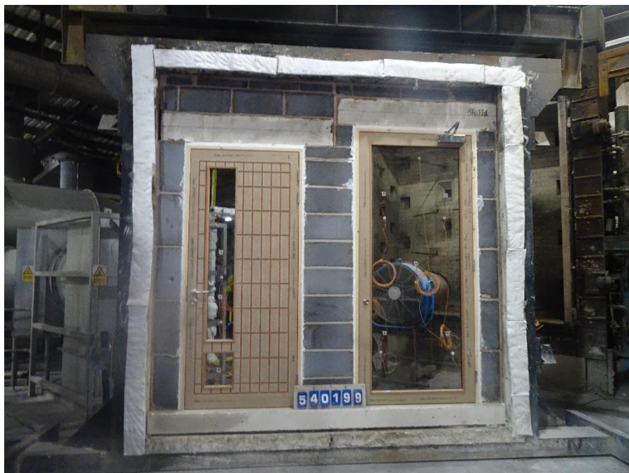
Figure 18 Exposed face of the specimen before the start of the test
