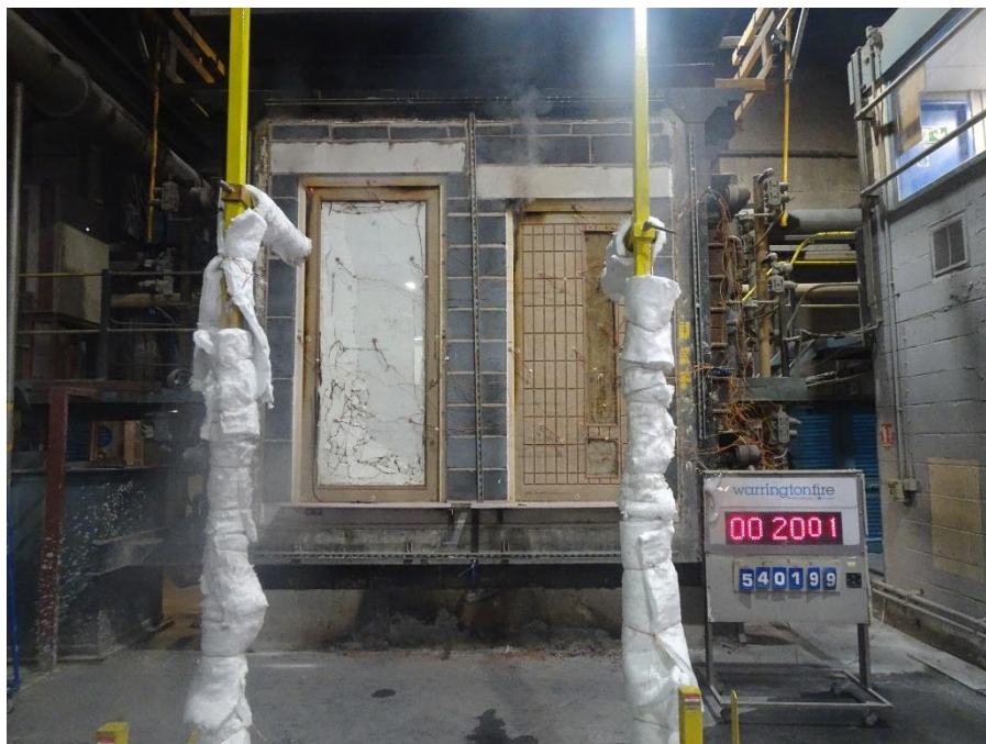
Figure 20 Unexposed face of the specimen at 20 minutes of testing
