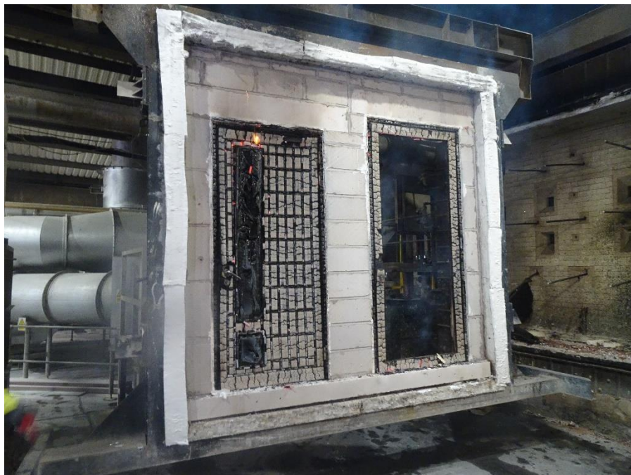
Figure 24 Exposed face of the specimen at the end of the test
