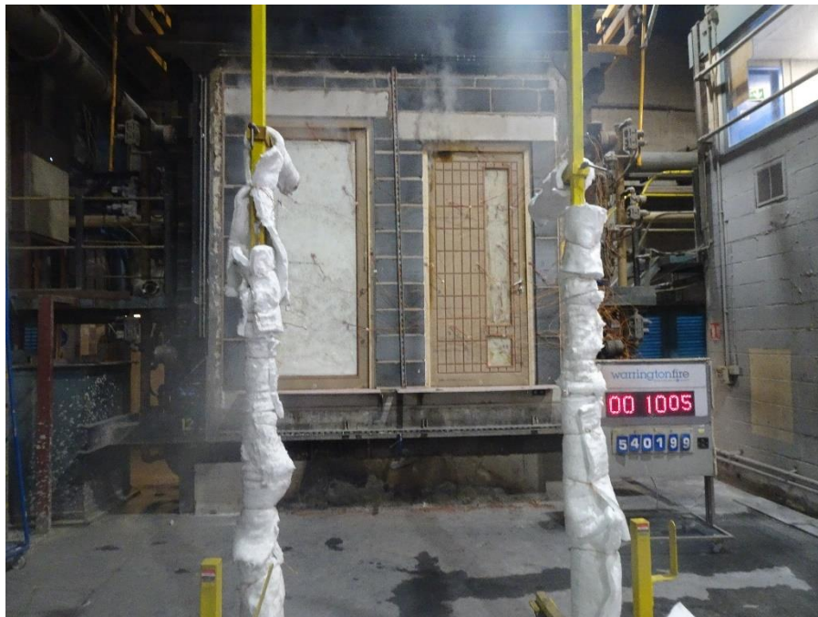
Figure 19 Unexposed face of the specimen at 10 minutes of testing
