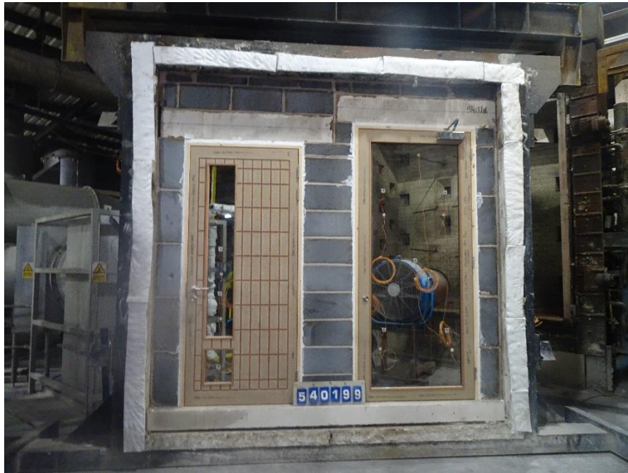
Figure 17 Unexposed face of the specimen before the start of the test
