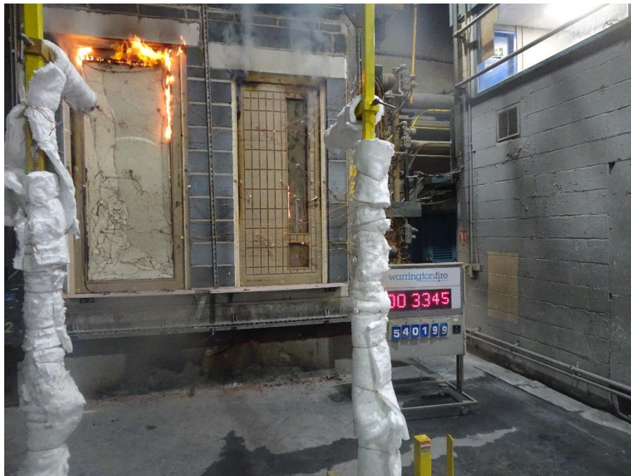
Figure 23 Unexposed face of the specimen at 33 minutes of testing showing sustained flaming up the edge of the glazing panel on Doorset B
