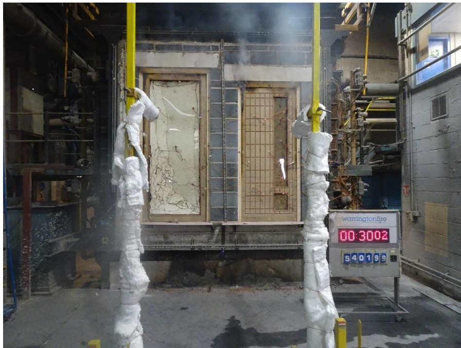
Figure 21 Unexposed face of the specimen at 30 minutes of testing
