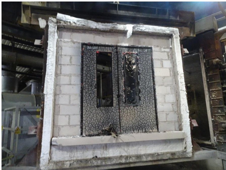
Figure 19 Exposed face of the specimen at the end of the test
