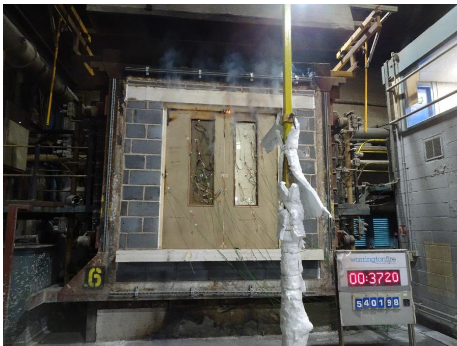
Figure 17 Unexposed face of the specimen at 37 minutes displaying sustained flaming
