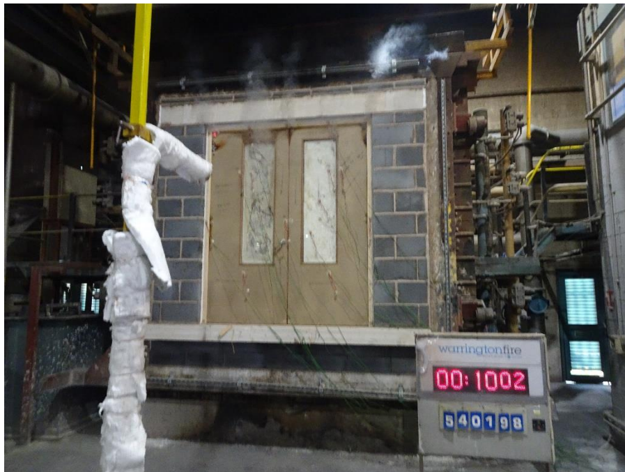
Figure 14 Unexposed face of the specimen after 10 minutes of testing
