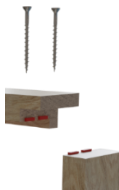
Trenched or Half Lapped Joint
