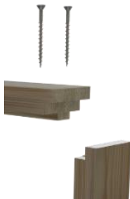
Half Lapped Joint
